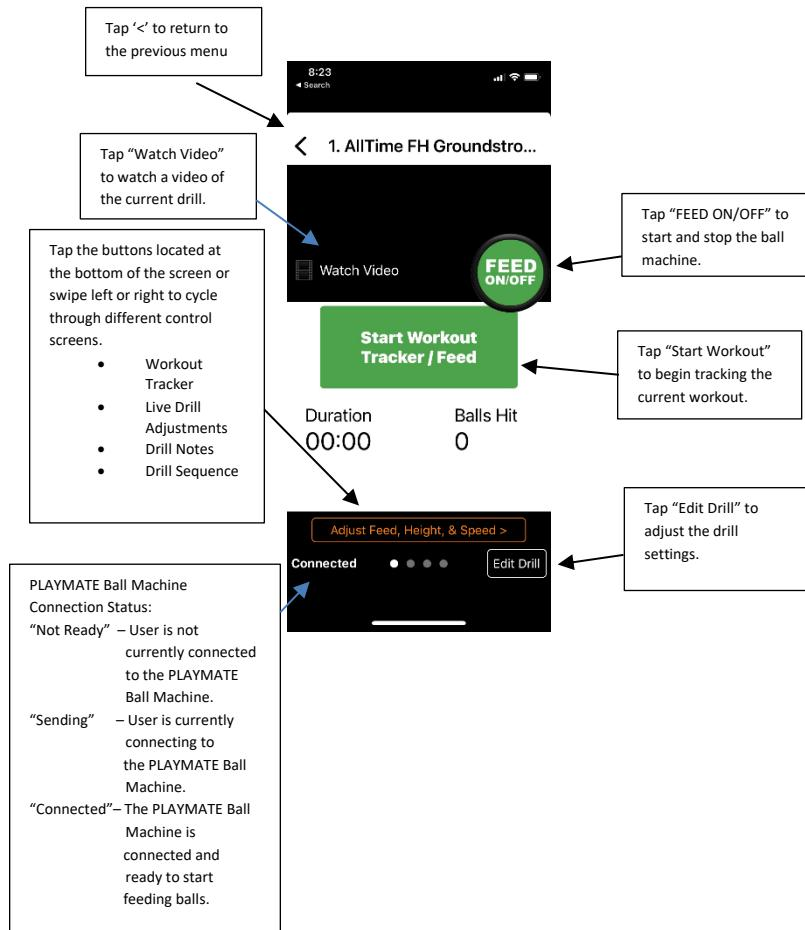
7. To start and stop the PLAYMATE Ball Machine during a workout, simply tap “FEED ON/OFF”.
