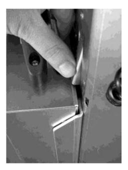
4. While pressing the battery-pack lock button, pull the batterypack up and out.
